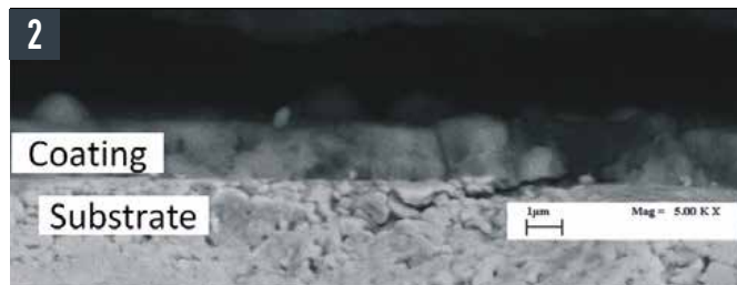
Fig. 2 • Cross-section of the coating after 2 hours of deposition
