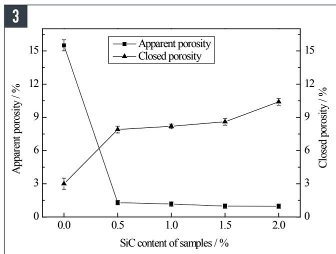
Fig. 3 • The apparent and closed porosity of samples with different amounts of SiC fabricated by the gelcasting method
