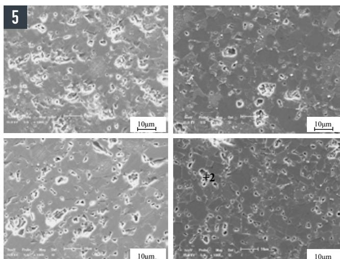
Fig. 5 • SEM images of fracture surface of samples fabricated by the gelcasting method
