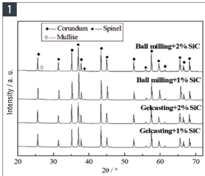
Fig. 1 · The XRD patterns of samples fabricated by two methods with various amounts of SiC
