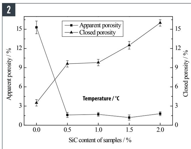
Fig. 2 · The apparent and closed porosity of samples with different amounts of SiC fabricated by the mixed ball-milling method
