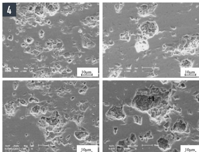
Fig. 4 • SEM images of fracture surface of samples fabricated by the mixed ball-milling method
