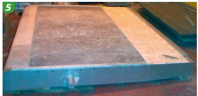
Fig. 5 • Aluminium furnace door with wear strip and heat shield
